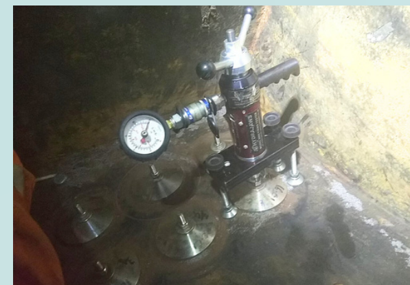
Proof load test of the C-Claw
