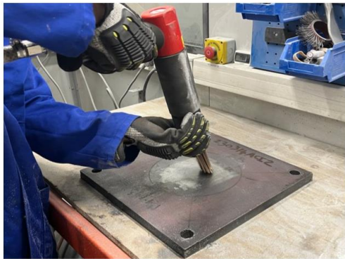
Optional coating removal with Needle Gun
