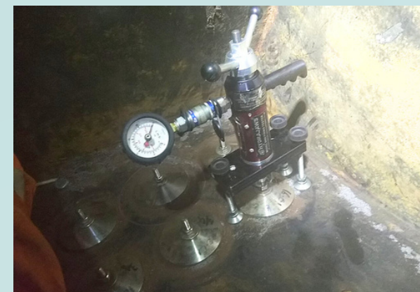
Proof load test of the C-Claw
